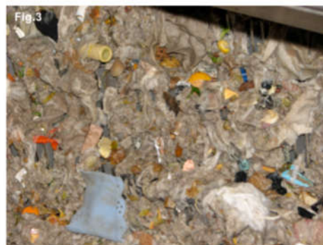
‘Screenings Filter Mat’ augments separation & removes hair, plastics & rags / wet-wipes
