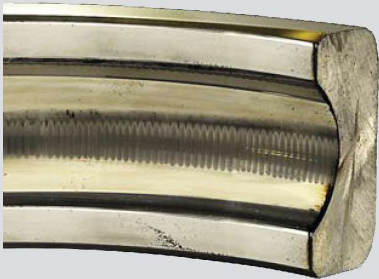
Bearing fluting, "washboard" pattern on bearing race
