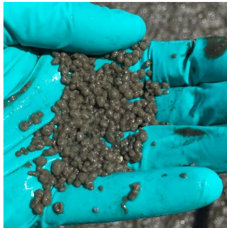
Figure 1. AquaNereda® Aerobic Granular Sludge
