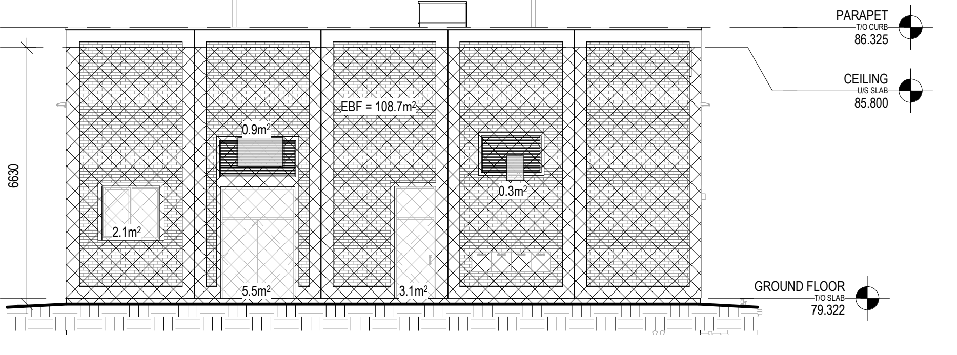
1 EXPOSED BUILDING FACE - EAST A4002 SCALE: 1:100
