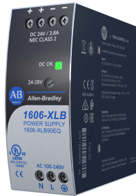
1606-XLB90EQ 3.8A (90 W) NEC Class 2 Screw Terminals
