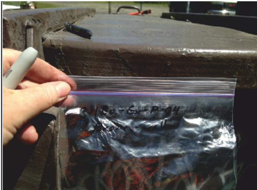
Photo 5: Bancroft Drive Lift Station Sample # 2811Ba-Ex-P- 04 – Well Cover (brown) - 2100 µg/g (0.21%) lead by dry weight – Condition - Fair
