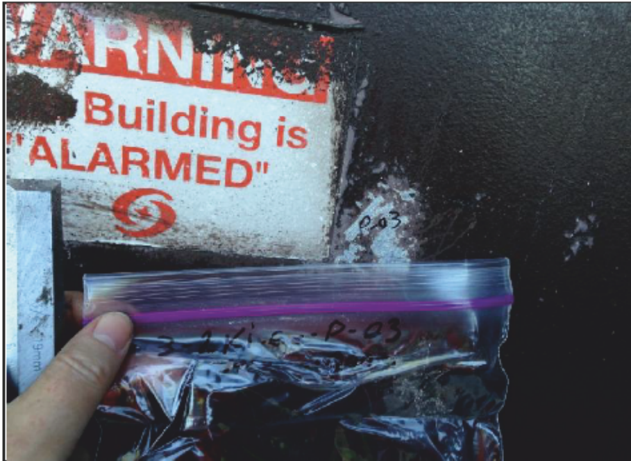
Photo 9: Kingsway Lift Station Sample # 1955Ki-Ex-P-03 – Entrance Door (Brown) - Result - <98 µg/g (<0.0098%) – Condition – Fair
